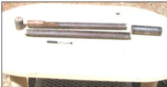
Photo (2) Standard Split spoon used for testing SPT.
