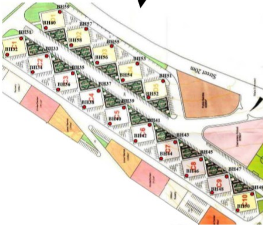
Fig (3) Site plan showing locations of the other fifteen apartment buildings with locations of the boreholes.
